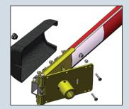
HyProtect breakaway arm bracket assembly.
